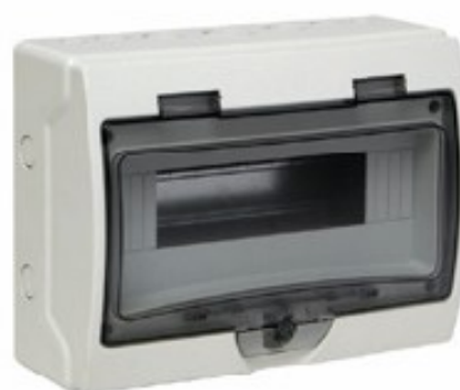
OPTION: IP65 BOX - 6 MODULES height (external): 200mm Width (external): 159mm Depth (external): 112mm Color: Light Grey IP65 Matter: Polystyrol
