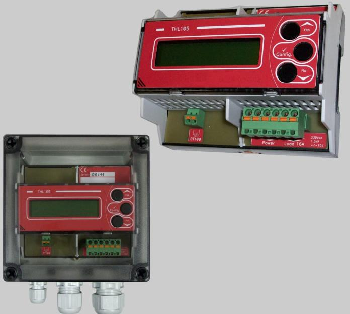
The THL105 is a compact field mount thermostat for regulating heating cables and ribbons, allowing control of resistive load up to 3.5 Kilowatts. The digital regulation allows to combine precision and ease of use. Temperature and set point are displayed on a large LCD display.
