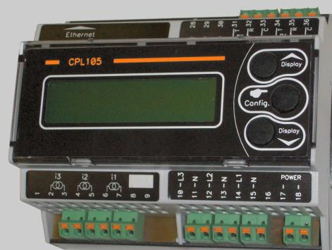
The CPL105 is primarily designed to measure power and energy in power management applications (management of buildings and workshops, ....), the Ethernet link allows measures supervision while ensuring easy and fast integration into existing networks. The internal bus allows multiple modules focused on Ethernet.
